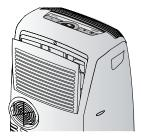
Use a vacuum cleaner to remove the dust collected on the filter. If it is very dirty, immerse in warm water and rinse a number of times. The water should never be hotter than 40°C. After washing, leave the filter to dry. Put the filter back in its housing.
