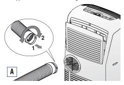
Screw the window outlet 17 to the other end of the exhaust hose. (see fig. B).
