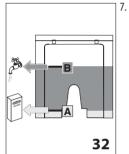
Pour the descaler into the tank up to level A (corresponding to a 100 ml pack) marked on the back of the tank (fig. 32), then add water (1 litre) up to level **B** (fig. 32) and put the water tank back.
