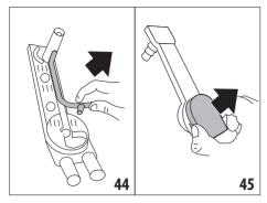
Extract the milk container (D7) from the thermal casing (D8);
