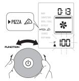
Turn the temperature/weight knob \$/\$\ilde{\Lambda}\$ (M) to set the weight of the pizza (from a minimum of 100g to a maximum of 900g)
