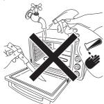
Make sure no water or liquid soap penetrates the vents on top of the oven.
