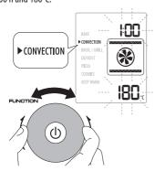
Turn the temperature/weight adjustment knob <sup>8</sup>/<sup>▲</sup> (M) to adjust the temperature (from a minimum of 80°C to a maximum of 220°C).
