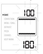
The values that can be changed, cooking time and temperature, flash. If these values are not set, the display will show 1:00 h and 180°C.
