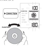
Turn the temperature/weight adjustment knob \$\mathbb{\bar{\sh}} \times (M)\$ to adjust the temperature (from a minimum of 80°C to a maximum of 220°C).
