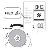
Turn the temperature/weight knob \$/\vec{\Left}\$ (M) to set the weight of the pizza (from a minimum of 100g to a maximum of 900g)
