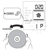
Turn the temperature/weight adjustment knob \( \bar{b} \) \( \bar{m} \) (M) to select the quantity of biscuits to be cooked: "1P" to cook biscuits positioned on a single level or "2P" to cook two levels at the same time.
