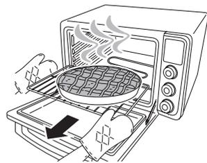
While CONVECTION function is running, it is possible to switch the function between BAKE and BROIL/GRILL without stopping the cooking process. Just turn the FUNCTION selection dial (O) to select the desired new function. Timer and set temperature will be kept between CONVECTION and BAKE. For BROIL/GRILL function, the timer will be kept and temperature is auto selected.
