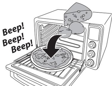
Close the door and complete the cooking process. At the end of the set time the appliance will play a sound signal and the display will show **00:00** flashing. The control is now in 'waiting mode'. In this state you can add up to 10 minutes, if necessary, to complete the cooking. This state is kept for 5 minutes, after that the control will turn off the oven automatically.
