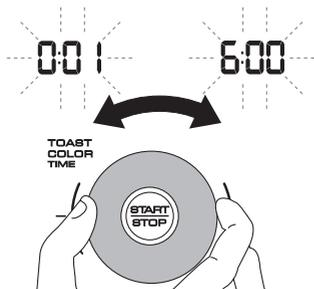
Press the START/STOP button (H) to start cooking. The red ON light (I), that is located around the edge of the START/STOP button (H), turns on.
