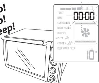
Turn the TOAST COLOR/TIME dial (G) to adjust up to 10 additional minutes, if necessary, and press the START/STOP button (H) at the end of time, the control will turn off the oven. To turn the appliance off during running function or reset the control at end of time when **END** is showed on display, press the START/STOP button (H) for 2 seconds. Open the door and remove the food. Take great care when taking the food out of the oven. Use oven gloves.
