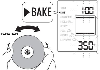
Turn the TEMPERATURE/PIZZA SIZE/SLICES/TRAY dial (M) to set the desired temperature. The default temperature is 350 °F.
