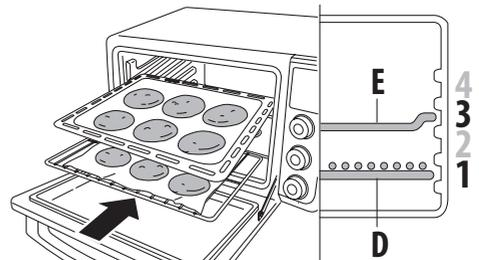
While in the 2 tray cookie mode the oven will beep 3 times. It is a signal to swap the trays, placing the top one on the bottom and vice-versa and press the START/STOP button (H).
