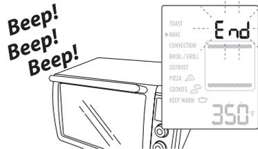
To turn the appliance off during running function or reset the control at end of time when *END* is showed on display, press the START/STOP button (H) for 2 seconds. Open the door and remove the food. Take great care when taking the food out of the oven. Use oven gloves.
