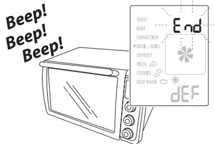
To turn the appliance off during running function or reset the control at end of time when *END* is showed on display, press the START/STOP button (H) for 2 seconds.
