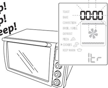
Turn the TOAST COLOR/TIME dial (G) to adjust up to 10 additional minutes, if necessary, and press the START/STOP button (H) at the end of time, the control will turn off the oven.
