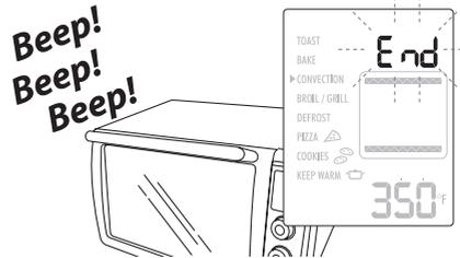
To turn the appliance off during running function or reset the control at end of time when *END* is shown on display, press the START/STOP button (H) for 2 seconds. Open the door and remove the food. Take great care when taking the food out of the oven. Use oven gloves.
