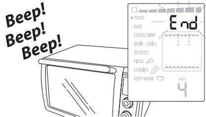
To turn the appliance off during running function or reset the control at end of time when *END* is showed on display, press the START/STOP button (H) for 2 seconds.
