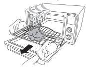
The bake pan located over the lower heating element works as fat container, collecting the fat or grease from grilled food. Carefully remove the bake pan and handle with care as you remove the fat drippings.
