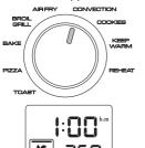
Turn the Time/temperature/toast color/pizza size/slices/tray dial (N) to set the desired time. The default time is 1:00 (hour), the default temperature setting is 360°F.
