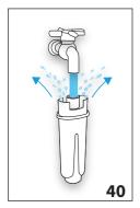
"RUN WATER INTO FILTER HOLE UNTIL IT COMES OUT" (fig. 40): To activate the filter, run tap water through the hole in the filter as shown in the figure until water comes out of the openings at the side for more than a minute. Press the selector corresponding to "NEXT>";
