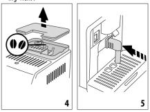
Insert the hot water spout (D6) on the accessories connector (A8) (fig. 5) and place a container with a minimum capacity of 200 ml under the coffee spouts (A7) and hot water spout (fig. 6);
