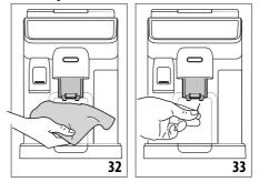
Check the holes in the coffee spouts are not blocked. If necessary, remove coffee deposits with a toothpick (fig. 33).
