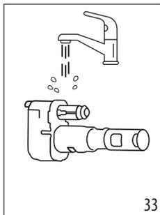
7. Rinse the milk carafe connector (E6) thoroughly (fig. 33). Take particular care to ensure that there are no milk residues in the air channel (see enlargement) (fig. 34): scrape the channel clean if need be, using a toothpick;
