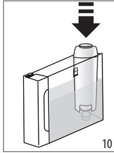
4. Insert the filter in the relative housing and press fully home (fig. 10);
