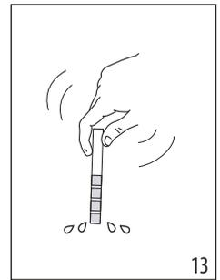
1. If a total hardness test strip (D1) is supplied with the model of machine in question, remove it from its wrapper.
