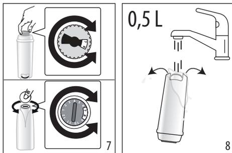
2. To activate the filter, run drinking water through the hole in the centre of the filter until water comes out of the openings at the side for more than a minute (fig. 8);
