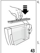
Remove the tank (A11) from the machine and fill with water. Insert the filter in the water tank and immerse it completely for about ten minutes, sloping it to enable the air bubbles to escape (fig. 41).
