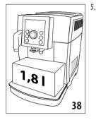
Pour the descaler (D3) into the tank up to level A (corresponding to a 100ml pack) marked on the side of the tank (fig. 36), then add water (1 litre) up to level B (fig. 37) and put the water tank back. Place an empty container with a minimum capacity of 1.8 litres under the coffee spouts (A17) and hot water spout (D6)(fig. 38).
