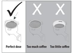
After grinding coffee for the first time, turn the dial (B2) gradually, starting from the "min" position (see following figure) until you reach the correct quantity, depending on the type of coffee. The ideal position is within the sector shown in grey in the following figure.
