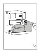
Empty the water tank (A8) completely and remove the water softener filter (C10) (if present).
