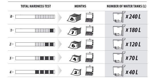
To determine descaling frequency, refer to the table (months of use or number of used tanks).
