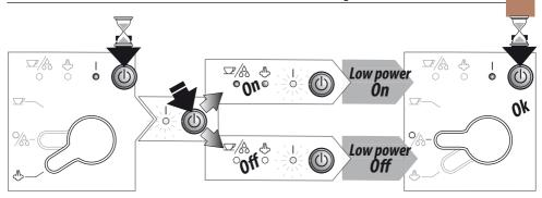
When LOW power is enabled, the device will automatically activate LOW POWER after 15 minutes and subsequently go into standby mode.
