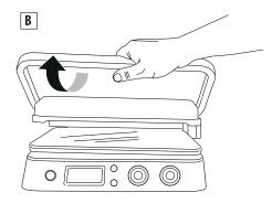
Lifting the upper plate further will automatically release the regulation system (fig. C).
