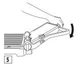
Lifting the handgrip slightly before pulling the release lever lightens pressure on the hinge and facilitates the operation.
